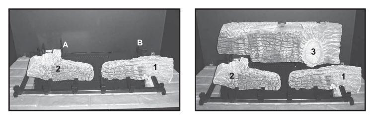
**STEP 4:** (SRV2057-722): Place log 3 so that the bottom notches mate with the 2 back steel tabs. Tab A is located on the right side of pilot bracket, tab B is located at the back/right corner of burner. NOTE: There should be a 1/2 inch gap between the bottom of log 3 and the top edge of the burner. The underside of log #3 must not cover ANY burner ports.
